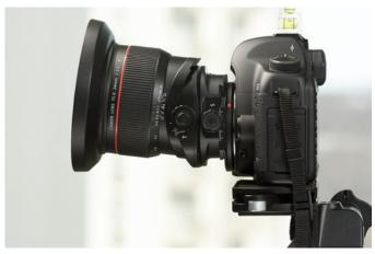
STATE OF THE ART tools, like this 'tilt-shift' lens (which allows precise control and correction of perspective and focus) enable specialist professionals to obtain images of the highest quality. Needless to say, this kind of equipment is not cheap. (See the 'The Specialist's Advantage' box on the next page.)
