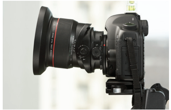
STATE OF THE ART tools, like this ‘tilt-shift’ lens (which allows precise control and correction of perspective and focus) enable specialist professionals to obtain images of the highest quality. Needless to say, this kind of equipment is not cheap. (See the ‘The Specialist’s Advantage’ box on the next page.)
